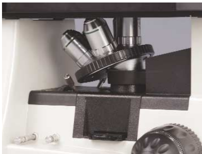
Close-up of the inverted nosepiece and objectives.
